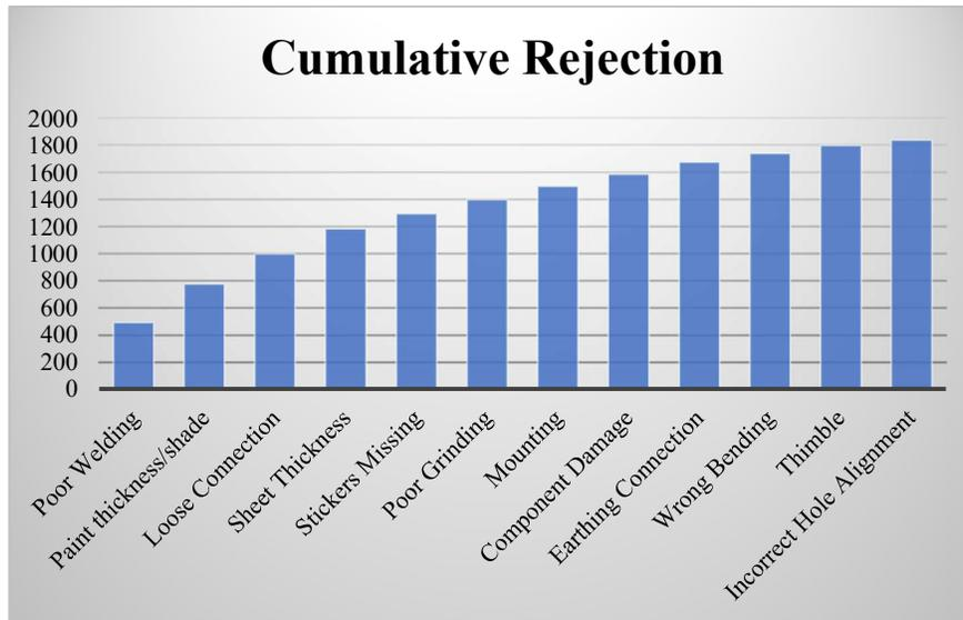
**Figure 5:** Trend of Cumulative Defect Rejection
